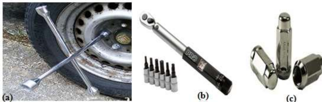
Fig. 1: (a) Spider-type lug wrench (b) Torque wrench (c) Spherical lug nut
