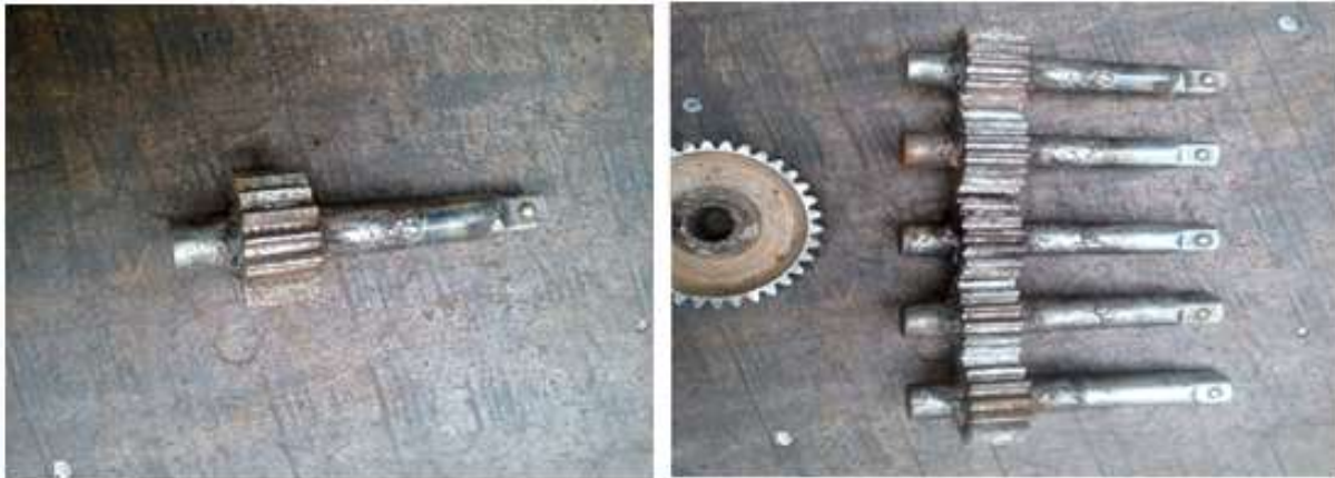
Plate 2: Shaft and Gear attachment with welding process
